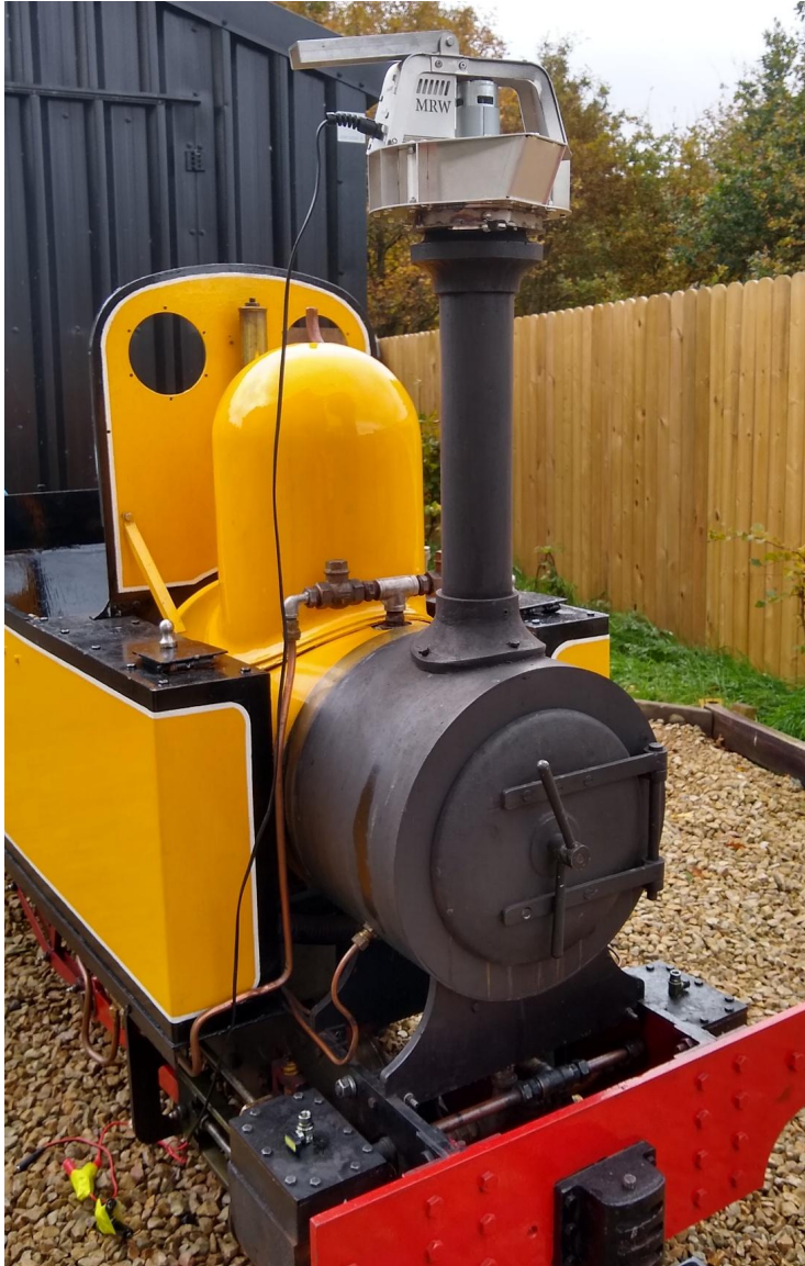
Hurricane blower in use with a Tinkerbell Class Locomotive.
