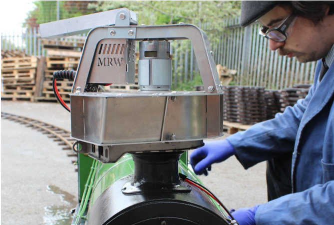
Hurricane Blower in use raising steam on a 7 ¼" gauge LNER K2.
