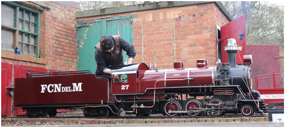
Hurricane Blower in use raising steam on the 9 ½" gauge Lakeshore Railroad
