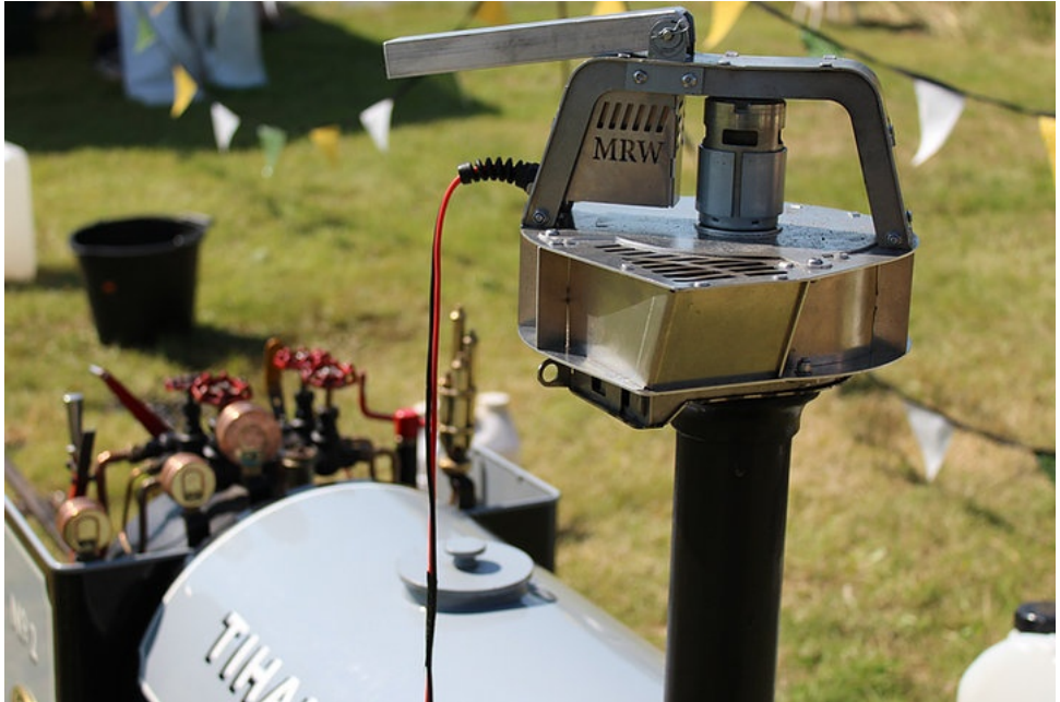
Hurricane blower in use with a Station Road Steam Stafford.
